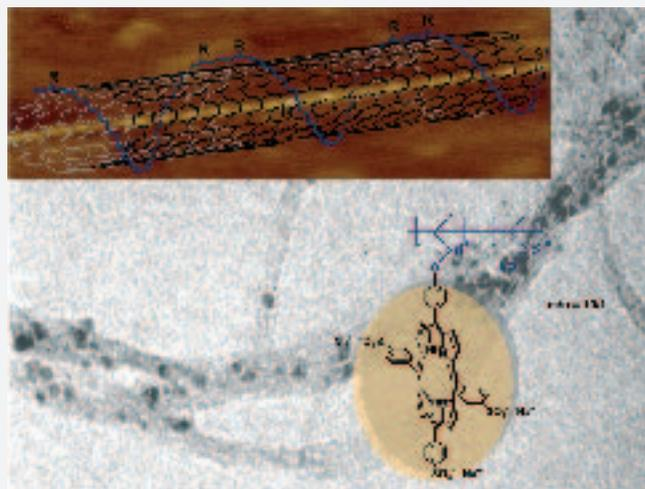
**Figure 5:** Leading example of a non-covalent approach (i.e., nanohybrids) towards the integration of SWNT as electron acceptor – together with free base tetraarylporphyrin ( $H_2P$ ) as light harvesting electron donor – into *electron-donor-acceptor* ensembles.
