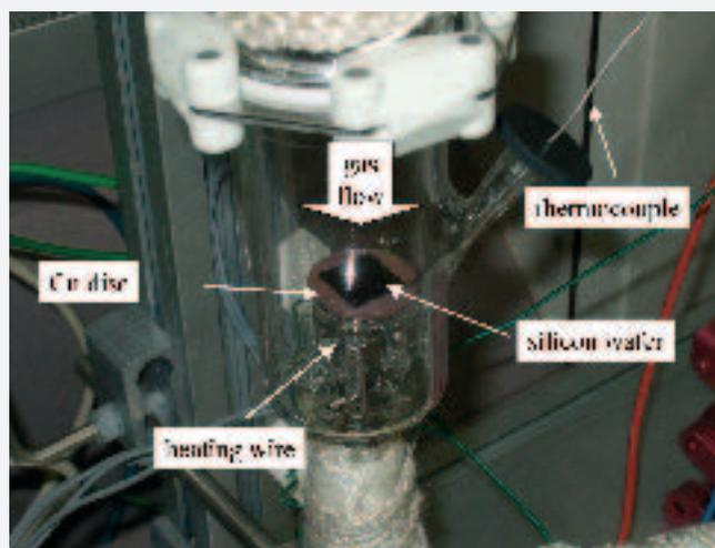
Figure 2. Coating of Si-wafer by MOCVD with **18** as precursor.
