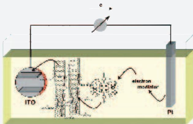
**Figure 6:** Schematic illustration of photocurrent generation in ITO-electrodes covered with a single SWNT • pyrene<sup>+</sup> • ZnP<sup>8-</sup> stack – red indicates baselayer of polyelectrolyte deposited initially onto ITO.
