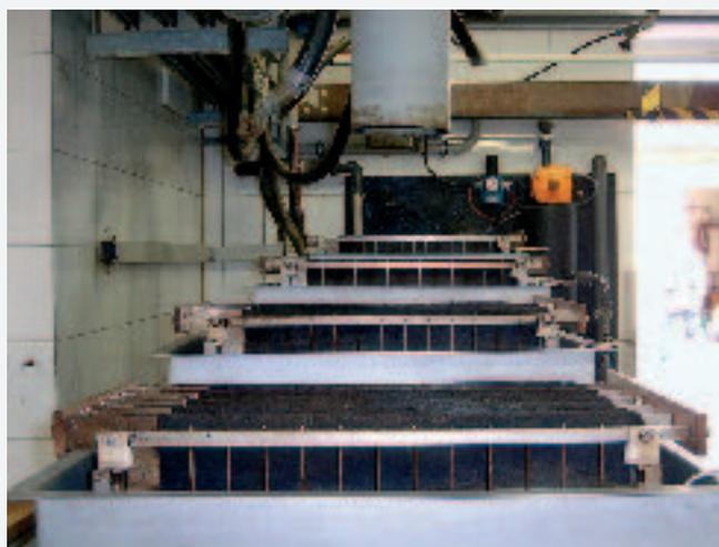
Fig. 3 Four electrochemical cells of a cascade with continuous flow.
