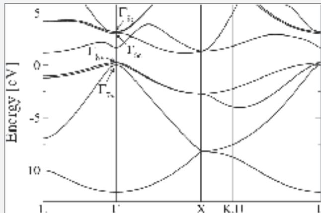
Fig. 6 EXX band structure of Ge including spin-orbit interactions (in eV).
