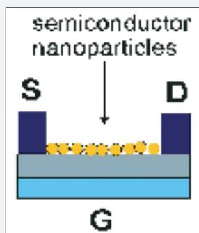
Figure 1: Field-effect transistor with source S, drain D and gate G.
