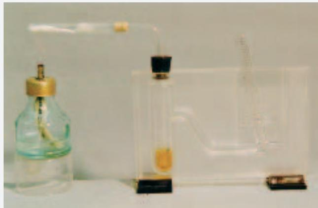
Cell K 1:  $\text{CaCO}_3 \rightarrow \text{CaO} + \text{CO}_2$
