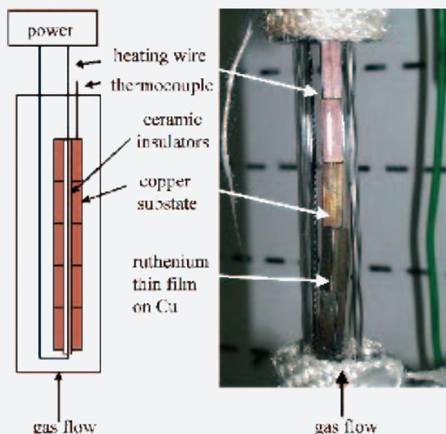
Figure 1. Coating of Cu-blocks by MOCVD with **17** as precursor.
