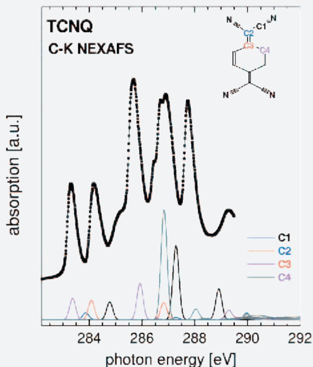
Fig. 1: High-resolution C K-edge NEXAFS spectrum from an ultrathin TCNQ film adsorbed on Ag(111) in comparison with ab-initio Hartree-Fock calculations for an isolated molecule.
