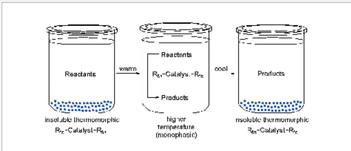
Scheme 6. Recovery of Fluorous Catalysts via Solid/Liquid Phase Separation.
