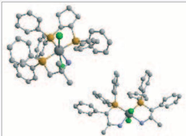
Figure 5. Perspective views of (a)  $\text{trans-[RuCl}_2\{(\text{S,S})\text{-C}_5\text{H}_8(\text{PPh}_2)_2\}(\text{Ph}_2\text{PCH}_2\text{CMe}_2\text{NH}_2)]$  (top) and (b)  $\text{trans-[RuCl}_2\{(\text{S,S})\text{-Ph}_2\text{PCH}(\text{Ph})\text{CH}(\text{Me})\text{NH}_2\}_2]$  (bottom).
