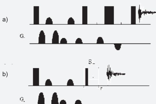
Fig. 1 Pulse sequence of a) DPGSE-NOE and b) DPGSE-ROE. SL denotes the (pulse-delay)<sub>n</sub> spin lock period, Gz denotes half-sinusoidal pulsed field gradients
