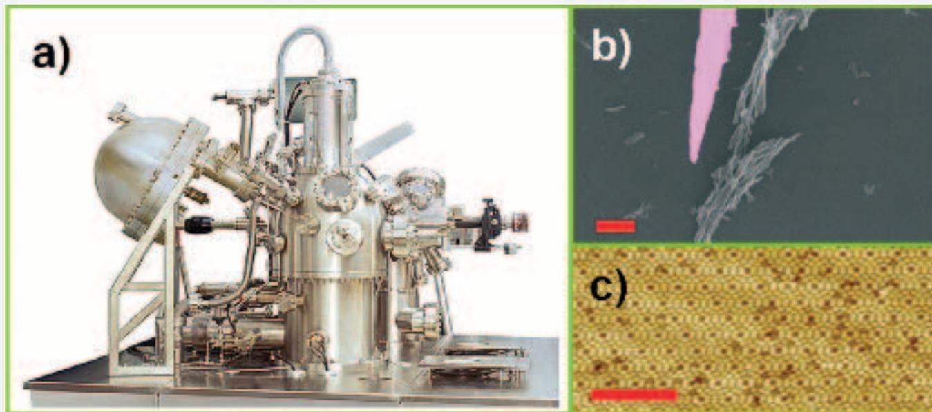
**Fig. 5:** a) Photo of UHV chamber with combined SEM, STM, and hemispherical electron energy analyzer (left).
