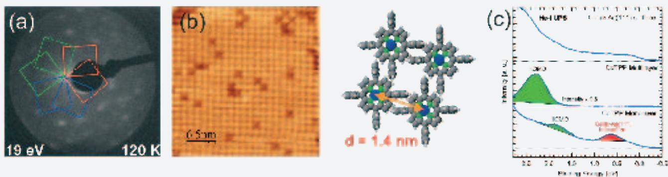
Fig. 1: Adsorption of Co(II)-tetraphenylporphyrin on a Ag(111) single crystal surface: (a) Low energy electron diffraction pattern of a well ordered monolayer; (b) corresponding scanning tunneling microscopy image of one of six nonequivalent domains, along with a schematic illustration of the lateral arrangement in the unit cell. (c) UV photoelectron spectroscopy data showing the valence region of the monolayer.
