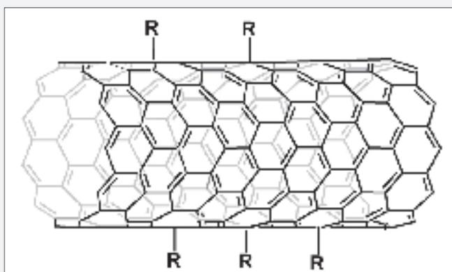
Figure 6: Sidewall Functionalized Carbon Nanotube
