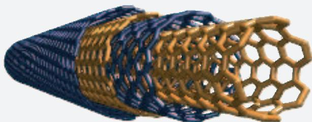
Figure 2: Carbon Nanotubes
