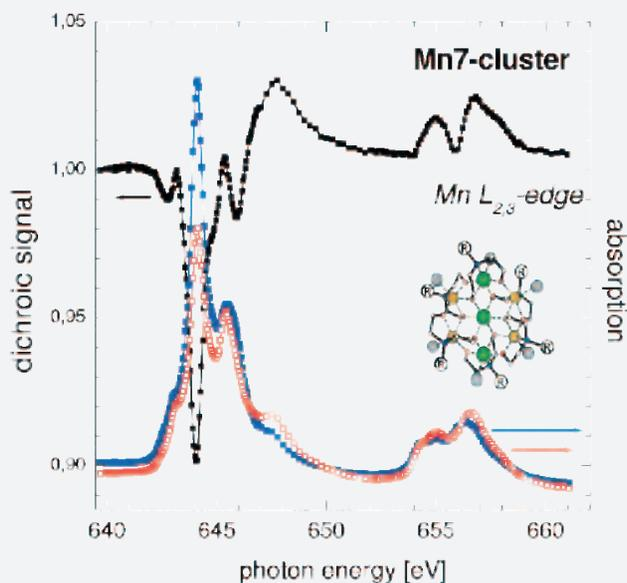
Fig. 2: Mn L<sub>2,3</sub>-edge NEXAFS spectra of supramolecules containing 7 Mn ions for circularly polarized light (blue, red) and corresponding XMCD spectrum (black). Spectra were collected at 10 K and a magnetic field of  $\pm 3$  Tesla.
