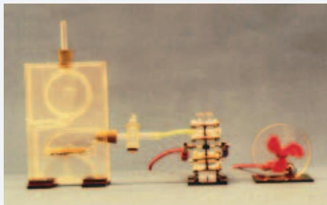
Cell K 3:  $\text{Zn} + 2 \text{HCl} \rightarrow \text{H}_2 \uparrow + \text{ZnCl}_2$
