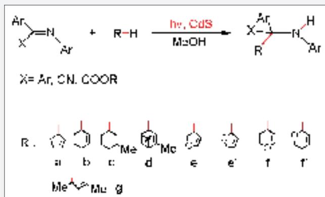
Figure 4: CdS photocatalyzed synthesis of homoallylamines.
