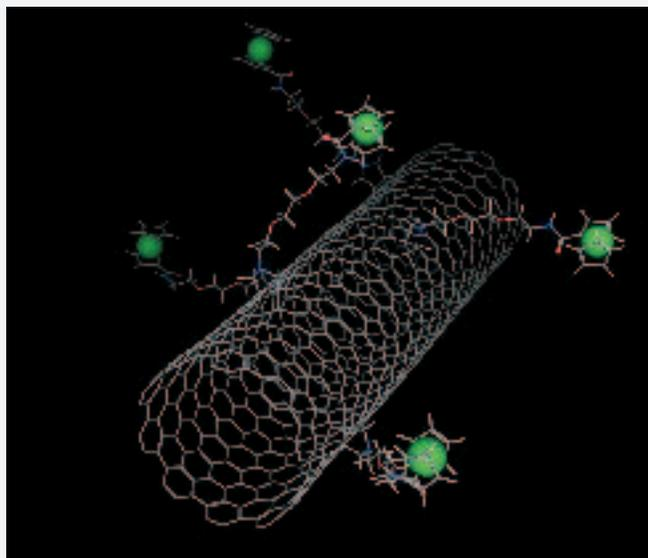
**Figure 4:** Leading example of a covalent approach (i.e., nanoconjugate) towards the integration of SWNT as electron acceptor – together with ferrocene electron donor – into *electron-donor-acceptor* ensembles.
