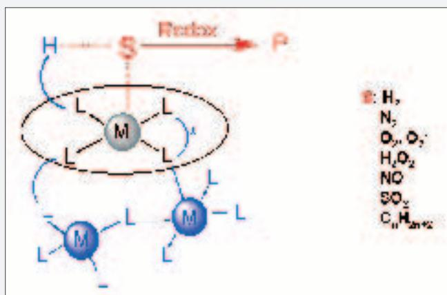
Figure 1: Activation of substrate S and redox transformation to P.
