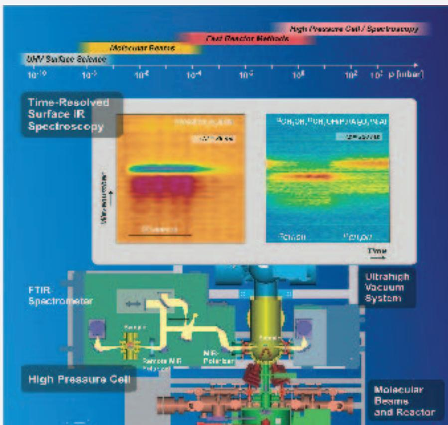
**Fig. 3:** (top) Kinetic and spectroscopic experiments on model catalysts can be performed from ultrahigh vacuum conditions to atmospheric pressure (IR spectra adapted from [2]). (bottom) Time-resolved surface IR spectroscopy in reflection absorption mode under ultrahigh vacuum conditions, in combination with molecular beams, fast reactor methods and a high-pressure cell using polarization dependent methods.
