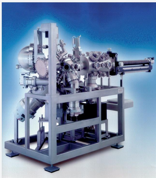
Fig. 3: Photo of a transportable UHV apparatus that combines high-resolution X-ray photoelectron spectroscopy (HR-XPS) and supersonic molecular beam. It is used for in situ studies of chemical reactions during adsorption and/or while heating the sample; the measurements are performed at synchrotron radiation facilities, e.g., BESSY II in Berlin [5]. Due to the high photon flux, full XP spectra can be measured within 1 second.
