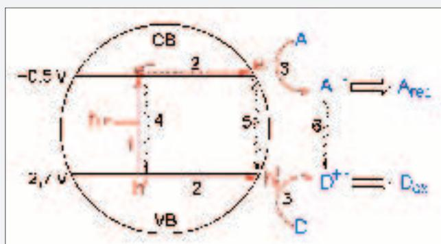
**Figure 1:** Schematic view of UV light driven photocatalysis at titanium dioxide. The circle symbolizes a particle, the two horizontal lines represent the upper and lower edge of the valence and conduction band, respectively.
