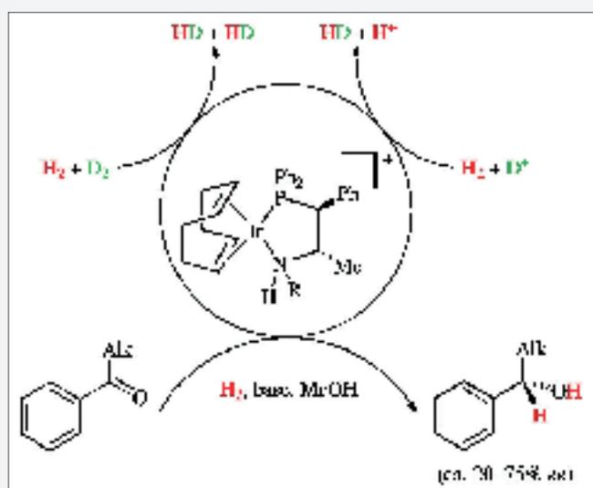
Figure 4. Catalytic >C=O hydrogenation and H<sub>2</sub>/D<sup>+</sup> and H<sub>2</sub>/D<sub>2</sub> exchange catalyzed by cationic [(COD)Ir{P<sub>2</sub>N(H)R}]<sup>+</sup> complexes.
