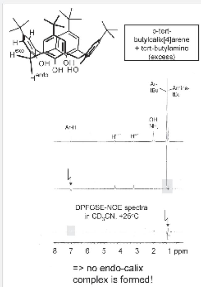
Fig. 2 NOE experiments on a mixture of tert-butylcalix[4]arene and tert-butylamine (excess). Top: normal  $^1\text{H}$ -spectrum. Middle and bottom: DPFGE-NOE spectra under irradiation at the indicated positions. Missing signals within the grey fields indicate remote entities and are not compatible with a claimed endo-calix complex.
